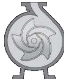
Expanding Volute Casing (Standard Pump)
